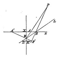
Then, as in Art. 2, any number of points on the curve may be obtained by taking successive positions of E on the directrix.
